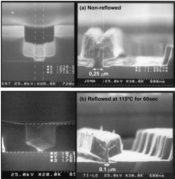
Fig. 1. Scanning electron microscopy micrograph. (a) Conventional e-beam resist and its 0.25- $\mu\text{m}$  T-gate. (b) The resist after shrinking by thermally reflow and its 0.1- $\mu\text{m}$  T-gate.
