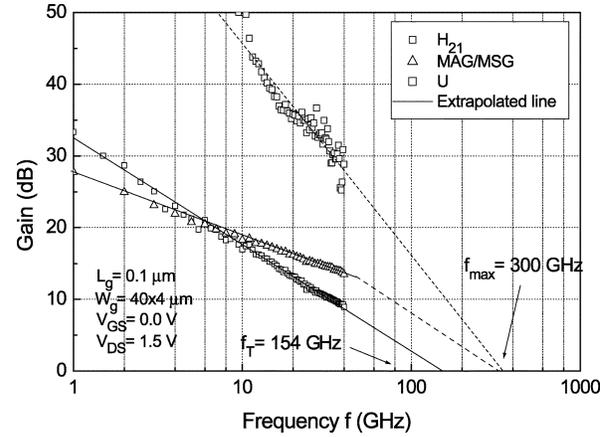
Fig. 3. Typical current gain  $H_{21}$ , MAG/MSG, and unilateral gain  $U$  as a function of frequency of the 0.1  $\times$  160  $\mu\text{m}$  MHEMT.
