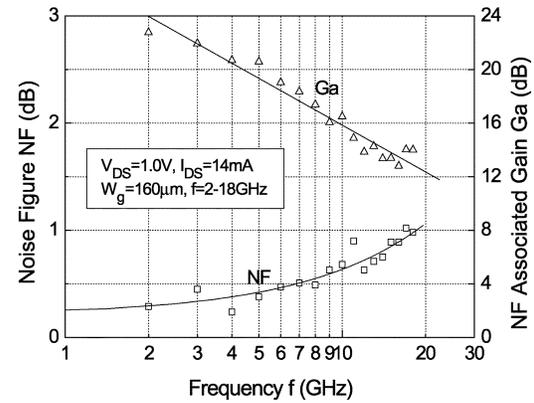
Fig. 4. Noise figure and associated gain as a function of frequency at  $V_{DS} = 1$  V and  $I_{DS} = 14$  mA of the 0.1  $\times$  160  $\mu\text{m}$  MHEMT.
