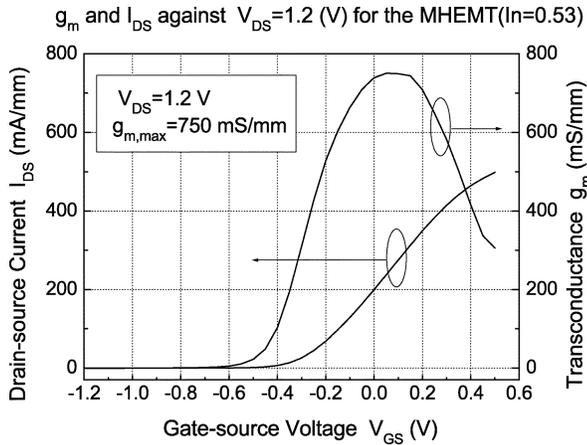
Fig. 2. Transconductance of the 0.1  $\mu\text{m}$   $\times$  160  $\mu\text{m}$  MHEMT.
