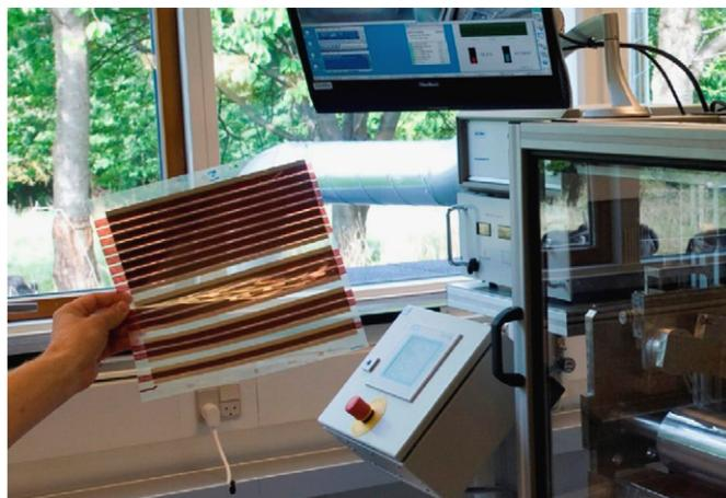
Fig. 8. Photograph of one of the final modules in front of the R2R coater.
