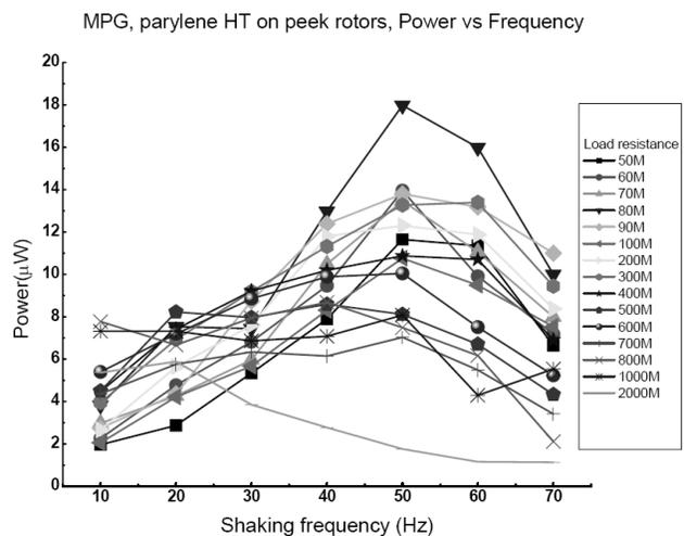
Figure 9. Power output with different load resistance versus frequencies.
