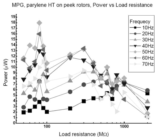
Figure 8. Power output at various frequencies versus load resistance.
