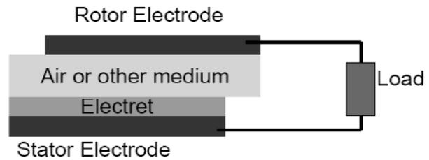
Figure 4. Conventional design of micro electret generator.
