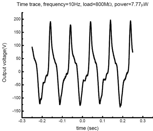
Figure 10. Output voltage at 10Hz with 800Mohm load.
