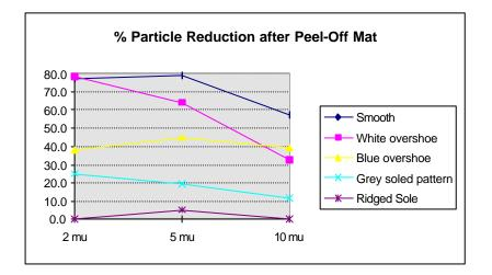
A comparison of performance of the two systems based on the average particulate reduction for all soling types is given in the table and chart below, which are largely self explanatory.
