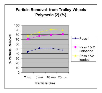
Particle counts are based on number per 10 cm2 of area of wheel (about half the complete wheel area). For this area, a removal of 8 to 10,000 particles per wheel on the double pass described is obtained. This approximates to 30 to 40,000 particles per trolley, per 10 cm2 of wheel area. Allowing for the actual wheel area, therefore, the number of particles removed will be approximately twice this figure at 60 to 80,000. **Table 10**
