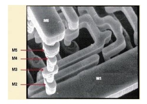
6 metal level copper dual damascene process crossection at 0.18µm node (R. DeJule, "Dual-damascene: overcoming process issues", Semiconductor International, pp. 94, June 2000)
