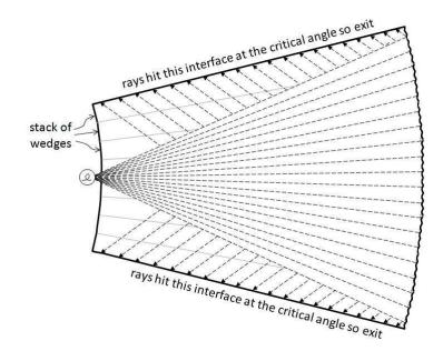
Fig. 3. Rays travel as if through a stack of wedges. The curvature of the thick end collimates the rays and the facets slew the direction of collimation so that rays illuminate the whole of the surface as they reach the critical angle.
