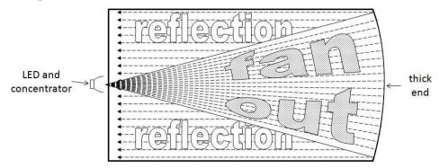
Fig. 1. Plan view: rays fan out to the thick end where they are reflected in parallel.
