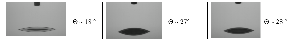
Figure1: Static contact angle ( \Theta ) of a water drop deposited on the untreated or pre-treated silicon (Si) substrate surface, DHB...dehydration bake
