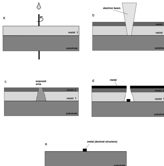
Fig. 1: Basic process steps in electron beam lithography
