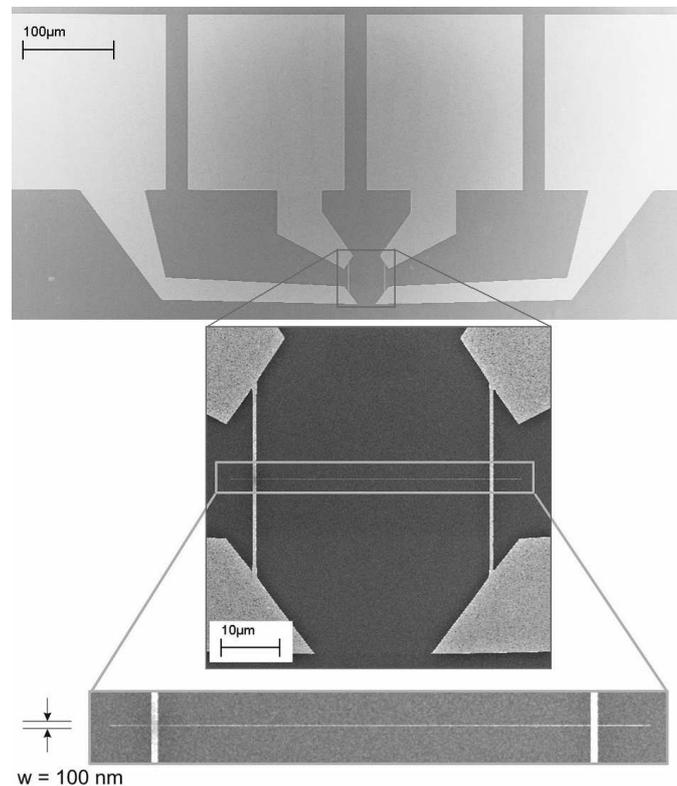
Fig. 5: Contacted nanowire prepared with a two step EBL process.
