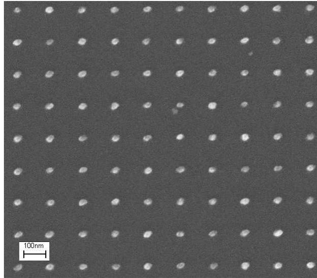
Fig. 2: Gold-dots with a diameter of  $\sim 35$  nm and a spacing of  $\sim 100$  nm on a silicon substrate.
