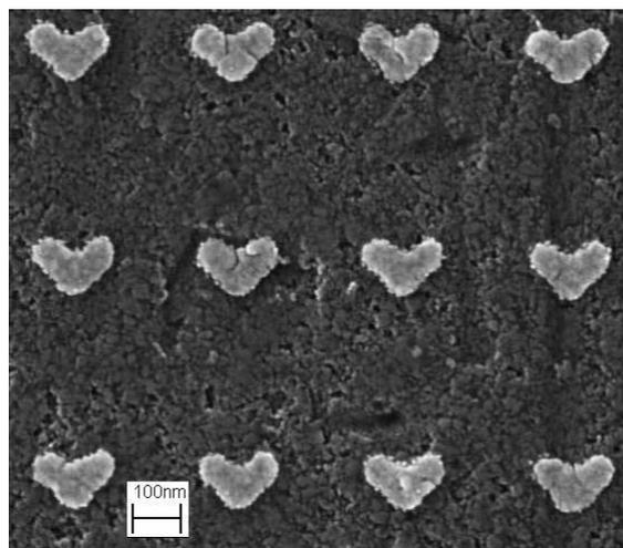
Fig. 3: Golden hearts on a quartz substrate covered with a 150 nm layer of ITO (indium tin oxide)
