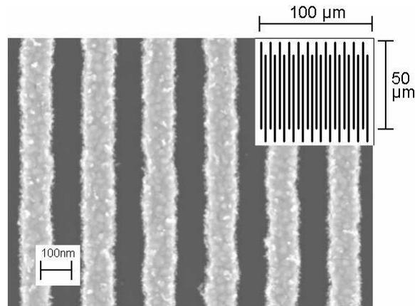
Fig. 4: An Array of gold nanowires with a width and spacing of  $\sim 100$  nm. The wires are 50  $\mu\text{m}$  long and the whole array has a length of 100  $\mu\text{m}$ .
